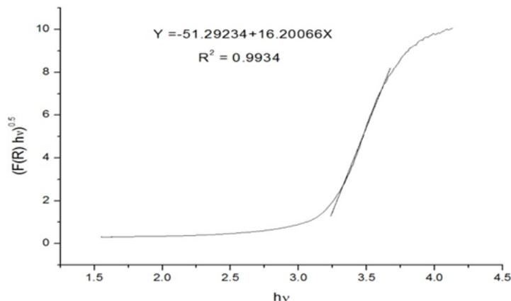
Figure 5. Kubelka–Munk Elaboration versus Energy for TiO<sub>2</sub> Powder
