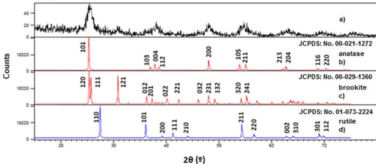
**Figure 1.** XRD Pattern of Synthesized  $\text{TiO}_2$  Nanoparticles
