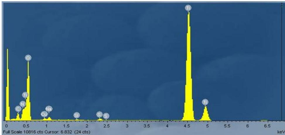
**Figure 3.** EDS Spectrum of TiO<sub>2</sub> Nanoparticles
