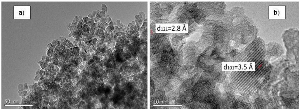
**Figure 4.** TEM Images of the Synthesized TiO<sub>2</sub> Nanoparticles
